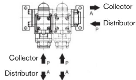
The SV modules with collector function have a non-return valve connected upstream as standard. As a result, the minimum pressure difference increases to 1 bar.
