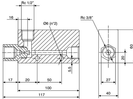
Single stage high suction power generators operating using a single large Venturi nozzle; particularly silent thanks to a free-flow silencer which is mounted separately. Suitable for use in dusty environments and in applications where a large suction capacity and a high degree of vacuum are required (92 -kPa).
