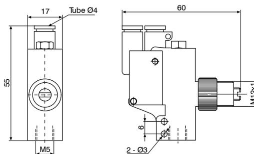
Vacuum switch whose function is, depending on the model, to turn a pneumatic signal on or off when a certain vacuum level is reached. The pressure differential that exists between the maximum value set and the restoration value cannot be adjusted. Especially recommended for the control of vacuum generators with a view to save energy.
