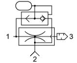
High-performance compact generator for high frequency applications; the presence of the integrated ejector ensures release capacity in the shortest possible time. The fact of it being extremely lightweight allows its application directly onto the robot gripping arms and/or mobile applications. Available with two flow rates in the same overall dimensions.
