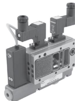
They have been designed to be enclosed between the cap and the base of the “SE” vacuum generator and attached to the latter via M4 screws; with the distribution manifold inside the generator, the compressed air is distributed without having to use external manifolds.
