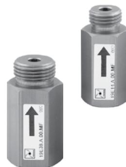
Non-return valves that can close the suction line in the event of air leakage from the suction cup that is not located on the workpiece or not fully adherent to it.
