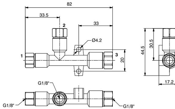
Single stage generators, robust and reliable, with compact dimensions and suitable for applications which need the required degree of vacuum to be reached quickly with limited air flows. Operating on the Venturi principle they have the vacuum connection orthogonal to the axis of supply and outlet. They can be connected directly to the suction cups and/or suction cup holder and applied in any position.
