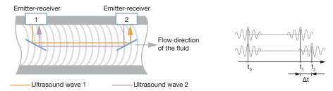
The electronic module delivers a pulse signal proportional to the volume or an industry standard 4...20 mA signal, proportional to the flow rate.
